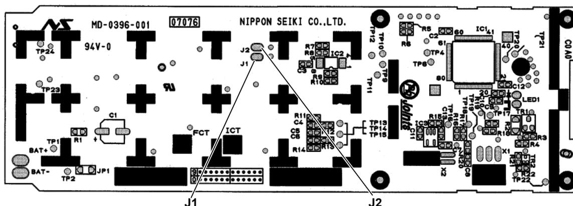
The P.C. board has the print "J1" and "J2". Solder "J1" and "J2" according to the number of indoor unit as shown in Table 1. After modification, press the RESET button.
