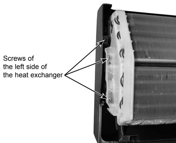
Screws of the left side of the heat exchanger
